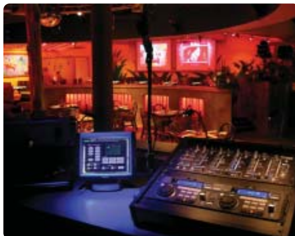
(Left) All presets are selectable from a Crestron TPS-3000 touchpanel located at the DJ position.
